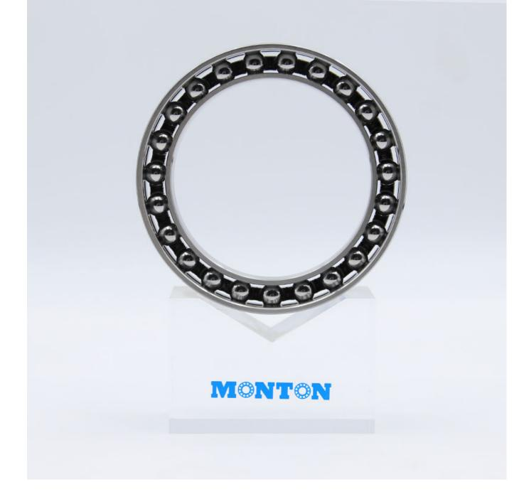
In the work of flexible bearing, the inner ring is installed on the elliptical cam, the outer ring is installed on the Flexspline, and the elastic deformation occurs with the rotation of the cam, which not only bears the cyclic stress load, but also bears the alternating stress load.
